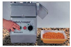
Using the vegetable preparation attachment of the Robot-Coupe R 602 V.V fitted with the  $5\times5$  mm brunoise accessory, cut the carrot, celeriac and courgette into dice.
