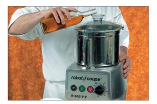
Make the dough for the tapenade pastry using the R 602 V.V. in its cutter mixer version, gradually increasing the speed from 300 to 1,500 rpm.
