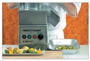
Using the R 602 V.V. in its vegetable preparation version, fitted with a 3-mm slicing disc, cut the baby courgettes into slices.
