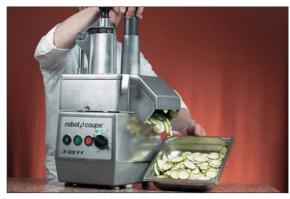
Using the Robot-Coupe R 602 V.V. in its vegetable preparation version, fitted with a 3-mm slicing disc, cut the courgettes, aubergines and tomatoes.
