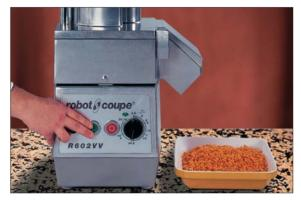
Again using the Robot-Coupe R602 V.V. in its vegetable preparation version, this time fitted with a dicing attachment  $(5 \times 5 \text{ mm})$ , cut the carrots into dice.
