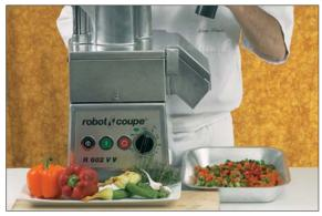
Using the R 602 V.V. in its vegetable preparation version, fitted with the dicing attachment (5  $\times$  5 mm), cut the red peppers and courgettes into dice.
