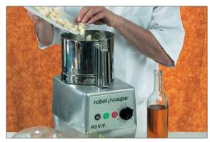
Using the R 3 V.V cutter, make the green and black olive crust, gradually increasing the speed from 300 to 1,500 rpm.
