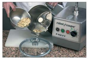
Using the R 602 V.V. in its cutter version, chop the almonds with the icing sugar, lemon peel, desiccated coconut and pistachios, gradually increasing the speed from 300 to 1,500 rpm.
